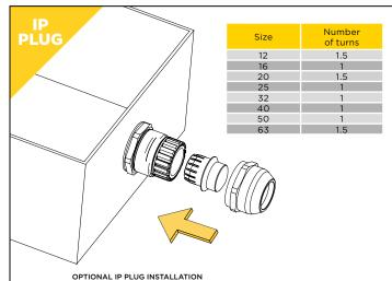
To install the IP Plug, insert the IP Plug as per the image (for the dual inner seals, make sure the notch in the IP Plug aligns with the tab on the seal) then tighten as per the table above.
