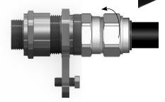
8. Connect the earth cable to the earth bolt.
