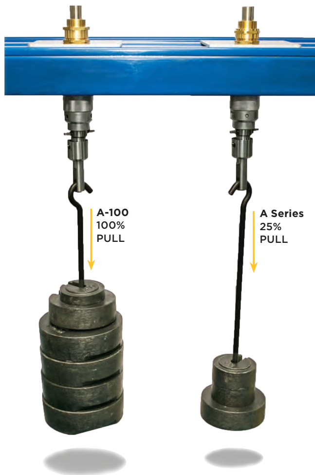
CMP A-100 and a standard A series cable gland during cable pull out resistance tests.
